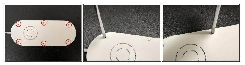
Remove the six 5 mm philips head screws.
