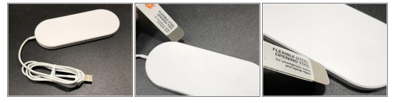
Turn the charger with the front up and insert a iSesamo between the gap.
