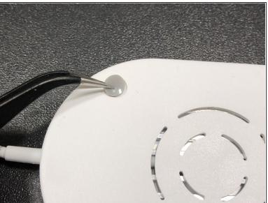
Remove carefully the six rubber feets from the housing with a tweezer.
