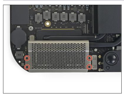
Use a T5 Torx driver to remove the four 2.8 mm screws securing the RAM shield.
