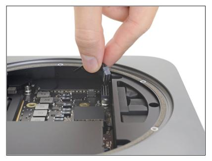
Grasp the power supply cable and lift to disconnect it from the logic board, wiggling as needed to loosen it up.
