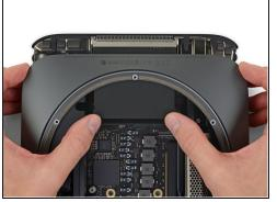
⚠ In this step, you'll push the logic board free from the clips holding it to the frame. **Push only where directed** or you may damage the fragile cooling fins.
