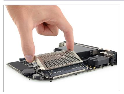
Lift the RAM shield and slide it off of the RAM assembly.
