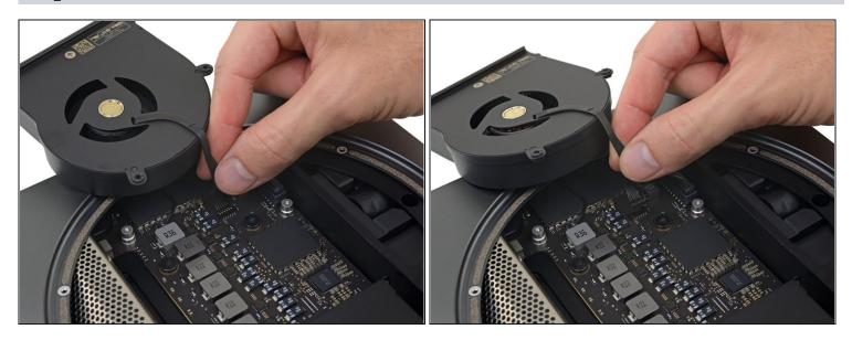
• Grasp the fan cable by all six wires and gently lift to unplug it from the logic board.
