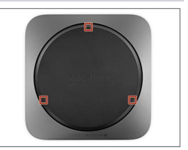
Lift and remove the bottom cover.
