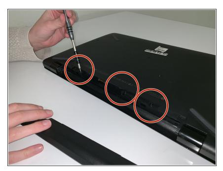
Use the Philips 0 screwdriver to unscrew the screws (7.51mm) that were underneath the battery.
