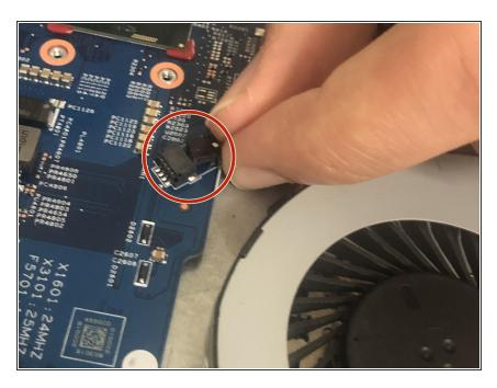
After removing the heat sink, disconnect the cable connecting the fan to the motherboard.
