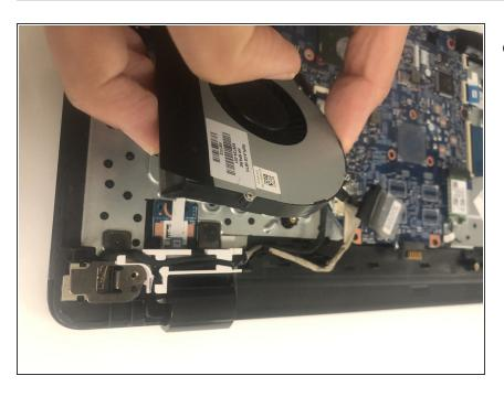
Remove the old fan from the device.
