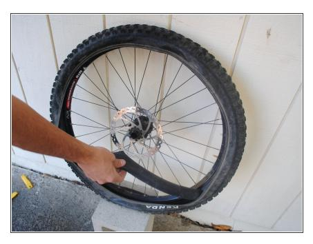
Using your hand, pull the tube completely out of the tire.
