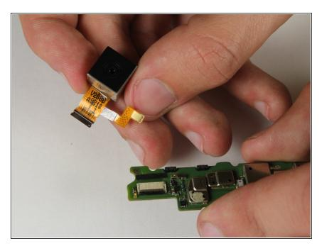
Reconnect the camera module by pushing the black end of the flat cable on the camera module into the white connector on the motherboard.
