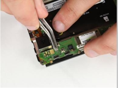
Carefully remove the white connecting wire from the motherboard using tweezers.
