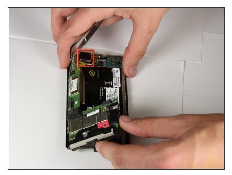
Carefully lift the motherboard and camera module up. Do not remove it from the phone!
