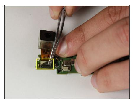
Remove the black electrical tape covering the cameras connection cable.
