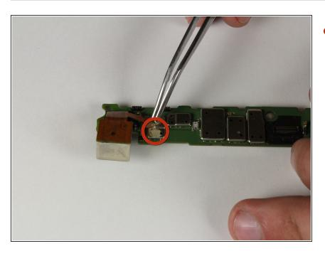
Gently peel the camera's orange and gold connection cable from the motherboard.
