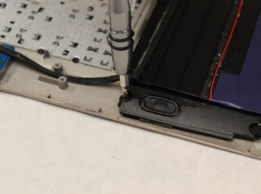
Unscrew the 4 1mm PH00 screws attaching the speakers to the frame.
