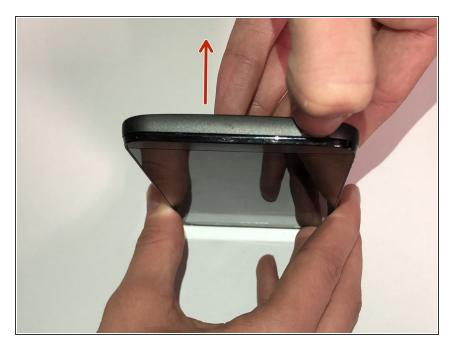
Pry the back cover from the bottom of the phone, pulling outwards and upwards.
