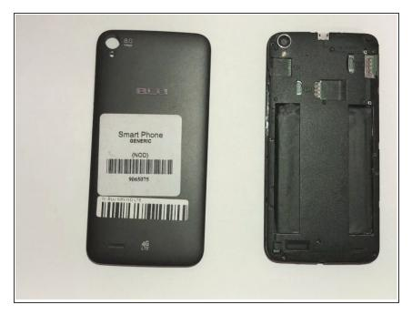
Fully remove the cover and set aside in a safe place.
