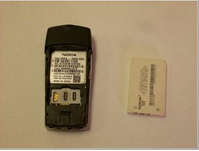
Use a screwdriver or spudger to lift the battery out of the casing.
