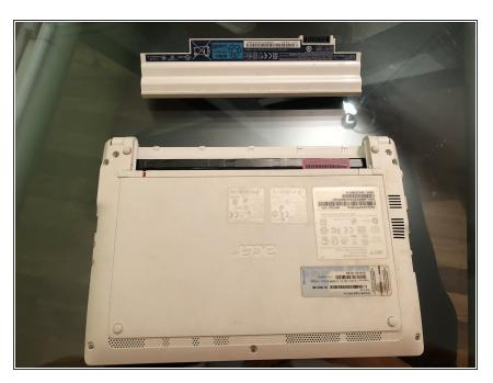
Remove the battery by pulling it out.
