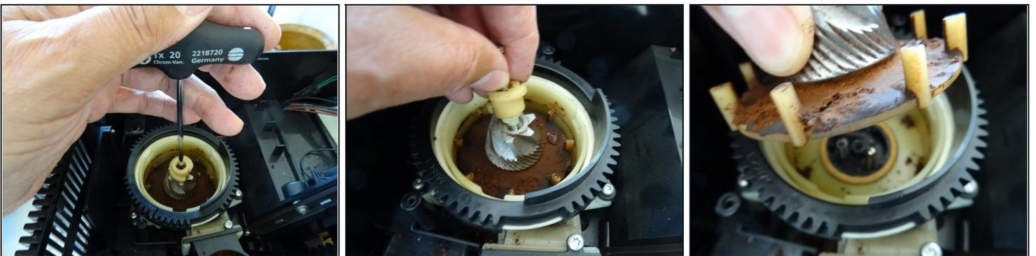
**⚠ In the next step be very careful not to loose these three springs, balls and cartridges.**
