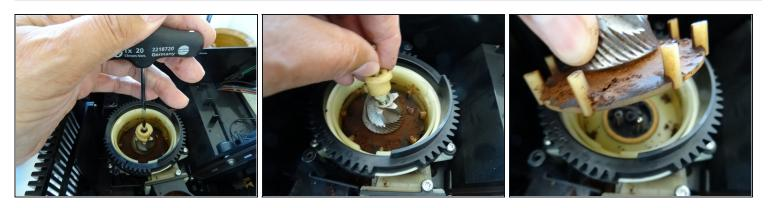
$\triangle$  In the next step be very careful not to loose these three springs, balls and cartridges.
