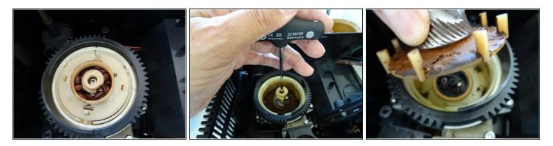
• Now the grinder is free. Again take a picture, then pull out the axis of the adjuster with moderate force.
