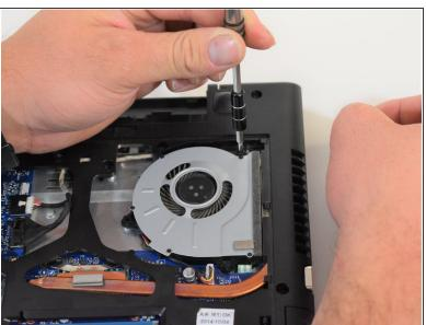
Remove the three 6mm Phillips #0 screws on the perimeter of the fan.
