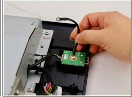
Detach the small black wire connecting the back metal plate to the USB video port by removing the one 8 mm Phillips #2 screw from the back metal plate and turning the screwdriver counterclockwise.
