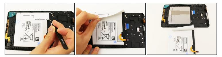
• Use the <u>tweezers</u> to lift the flap on the left end of the battery and pull up with your hand to remove the battery.
