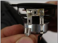
• Press the small metal tab on the speaker connector with a Phillips #000 screwdriver and gently pull the connector apart.
