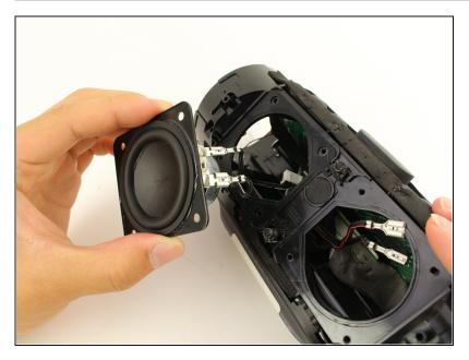
Now that the second speaker is disconnected from the motherboard, pull the speaker and wires out of the housing.
