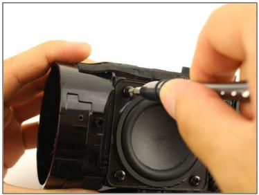
• Remove the eight 10mm Phillips #1 screws from around the two front speakers.
