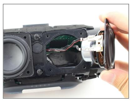
Pull gently on one of the speakers so it is outside of the housing. Be careful as it is still attached with the wires to the motherboard.
