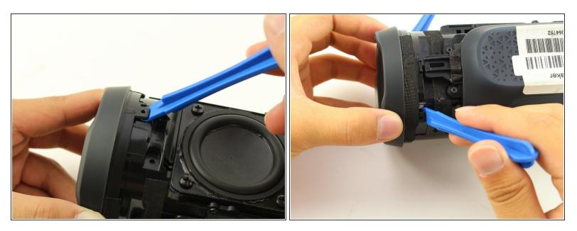
• Insert the plastic opening tools underneath both tabs.
