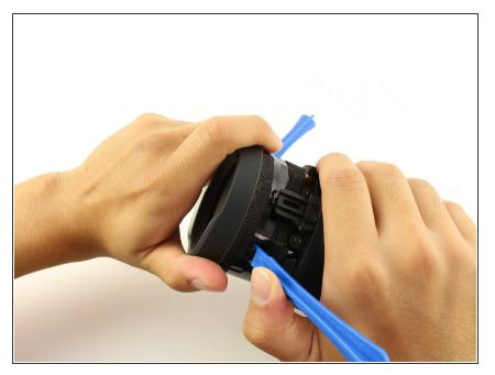
Twist and pull open the passive radiator. The left radiator twists off clockwise; the right counterclockwise.
