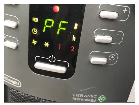
• Heater unit bricked with PF error (fault temperature sensor)
