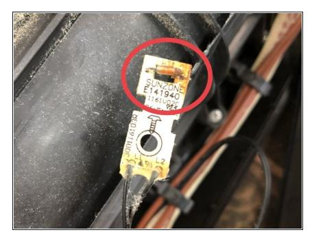
The temperature sensor had broken because it was corroded by moisture.
