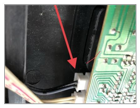
• Unclip the temperature sensor connector from the motherboard.
