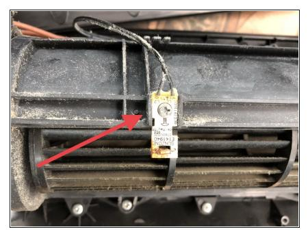
• Unscrew the Phillips screw to remove the temperature sensor.
