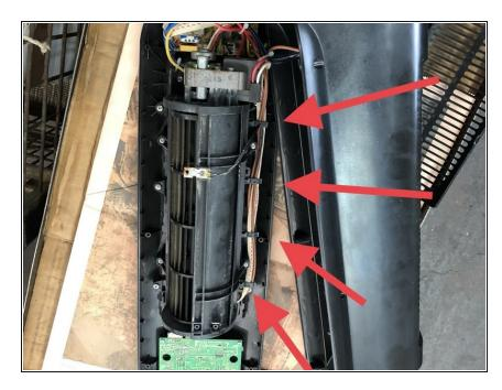
Open the clamps by unhooking them with pliers or using a flathead screwdriver.
