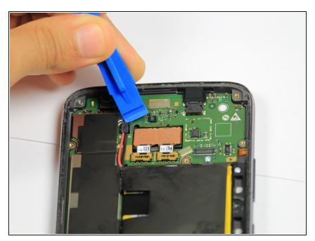
Use the opening tool to disengage the black connector located above the battery.
