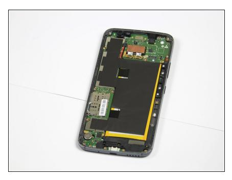
The battery is now fully exposed and ready to be removed.
