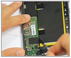
• Using the spudger, cut downwards along the black tape on left side of the battery.
