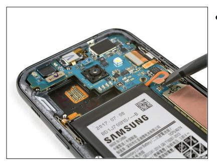
• Use the flat end of a spudger to disconnect the battery flex connector.
