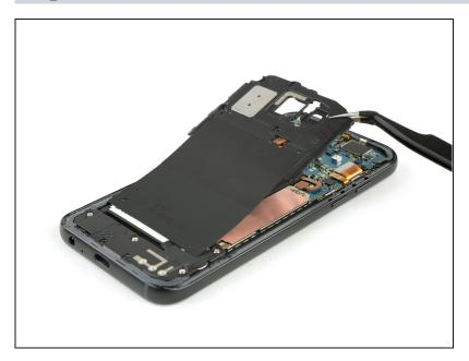
• Use a pair of tweezers to lift up the motherboard cover including the loudspeaker and the NFC antenna and remove it.
