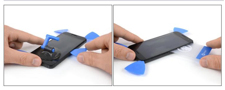
The screen's flex cable is located right behind the volume buttons, and may interfere with your cutting tool.
