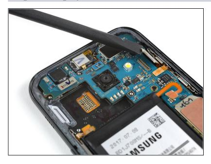
• Use the flat end of a spudger to disconnect the display flex cable.
