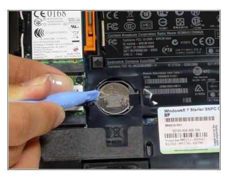
Pry the CMOS battery out with a plastic opening tool.
