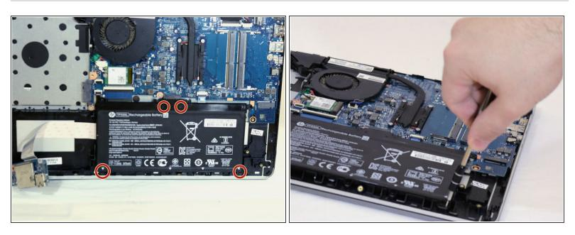
• Use a PH000 screwdriver to unscrew the four 3.5mm Philips head screws located on the battery.
