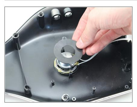
Lift the speaker retention bracket up and off the speaker.
