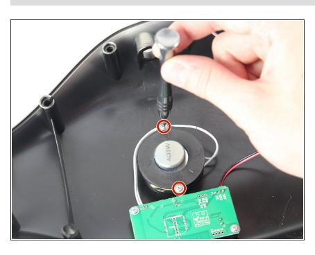
Remove the two 13mm Phillips #1 screws fastening the speaker retention bracket to the shell.
