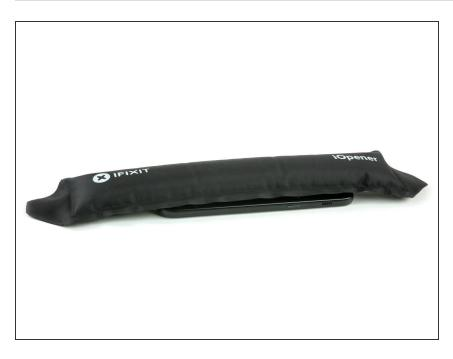
Use an iOpener to loosen the adhesive beneath the battery.
