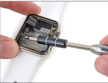
• Use a Y000 driver to remove the single tri-point screw securing the Force Touch sensor connector cable.
