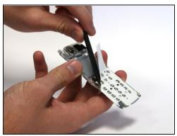
• Use the spudger to peel back the top-left corner of the white adhesive film. This can be done by working the spudger back and forth underneath the film.
