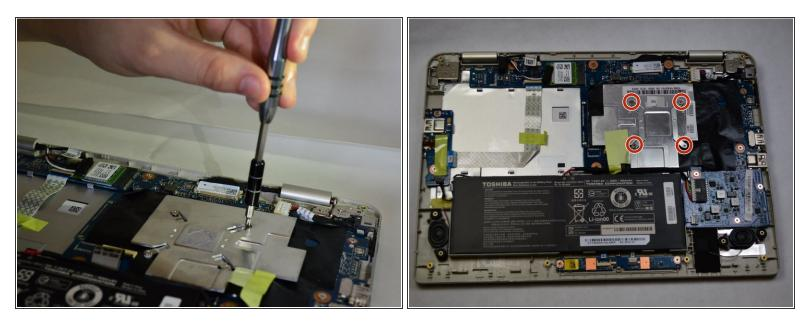
• Unscrew the four 3mm screws with the PH1 screw head, on the corner of the heatsink.
