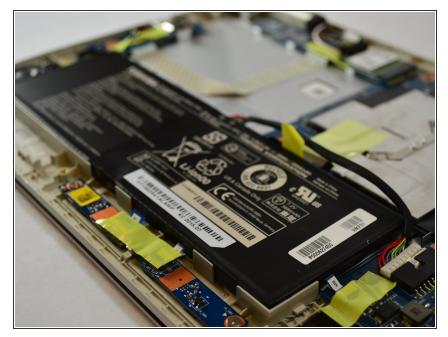
• Remove the 1" yellow tape on top of the battery. This piece of tape is holding down the battery connection cable.
