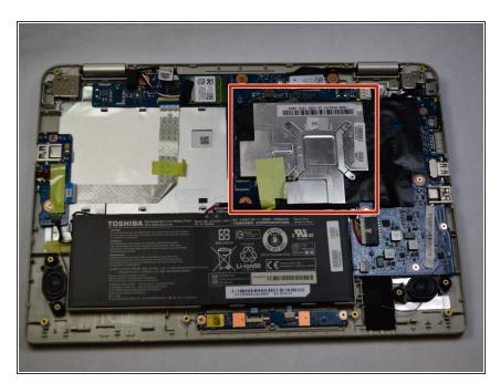
• Carefully remove the Heatsink from the board.
