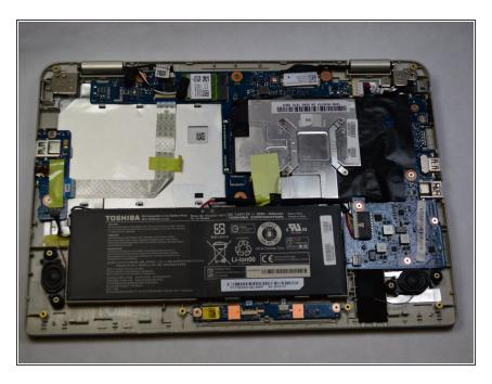
• Carefully pick up and remove the motherboard.
