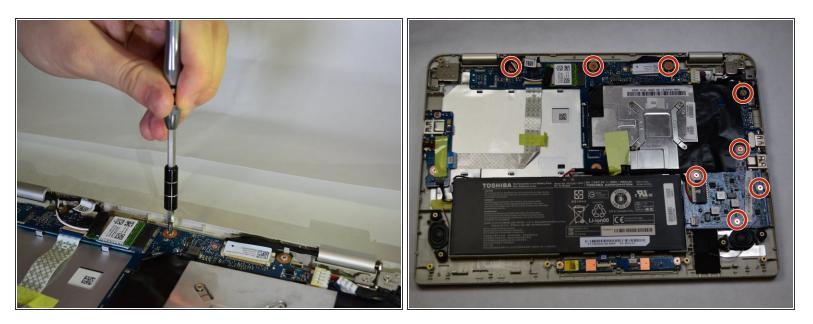
Unscrew the seven 3mm screws with the PH1 screw head, which are surrounded by a red circle to make identification easier, from the motherboard.
