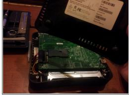
There are five Torx T10 screws holding the bottom to the top: one on each corner and a fifth underneath that "Warranty void if broken" seal. Unscrew all of them.
