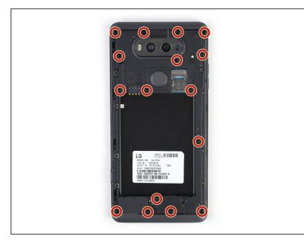
Remove the sixteen 4mm Phillips #00 screws attaching the back cover to the motherboard.
