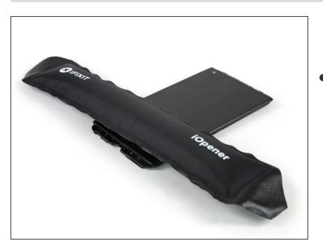
Use an iOpener to loosen the adhesive beneath the headphone jack and its flex cable.
