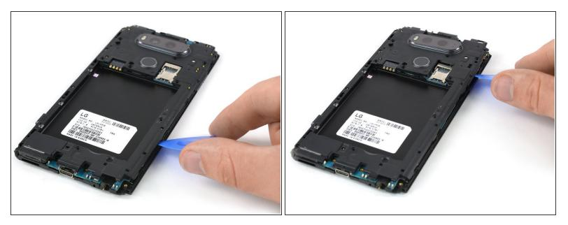
• Slide the opening pick along the mid frame and flip it sideways to open the plastic clamps holding the motherboard cover in its place.
