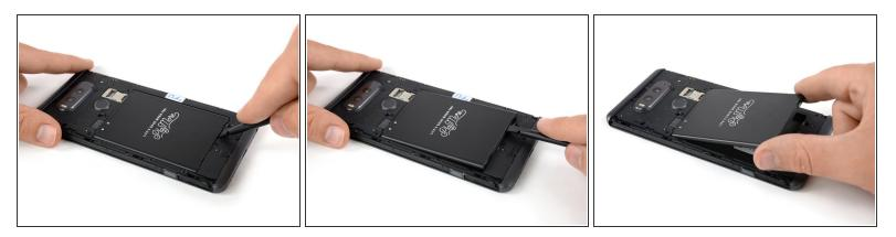
A Before disassembling your phone, discharge the battery below 25%. A charged lithium-ion battery can catch fire and/or explode if accidentally punctured.
