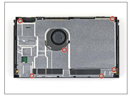
Use a JIS 000 screwdriver or an official iFixit PH 000 driver to remove the six 3 mm screws securing the shield plate to the device.
