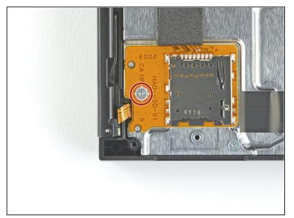
Use a JIS 000 screwdriver or an official iFixit PH 000 driver to remove the 3.1 mm screw securing the microSD card reader to the device.
