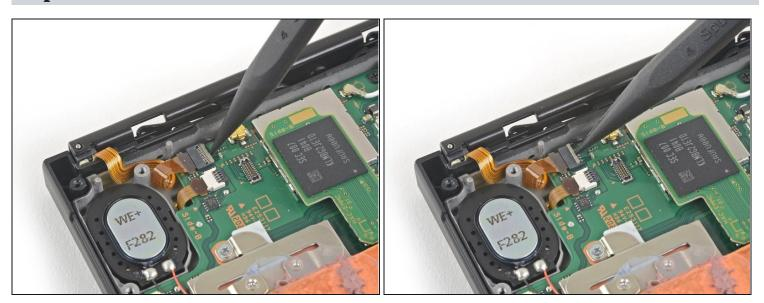
Use the point of a spudger, an opening tool, or your fingernail to flip up the small, hinged locking flap on the Joy Con sensor rail's data cable <u>ZIF connector</u>.
