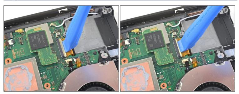
• Use an opening tool, spudger, or your fingernail to flip up the small, hinged locking flap on the LCD ribbon cable <u>ZIF connector</u>.
