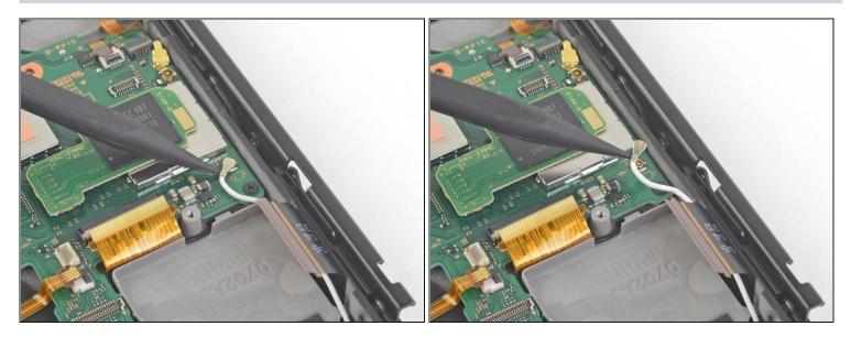
• Use the point of a spudger to pry up the white antenna cable straight up out of its socket on the motherboard.
