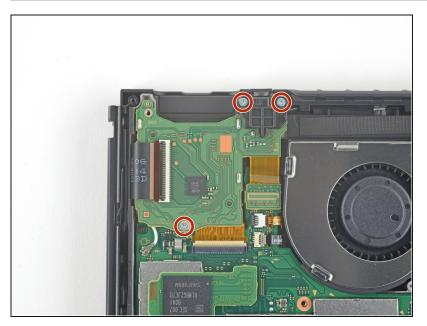
Use a JIS 000 screwdriver or an official iFixit PH 000 driver to remove the three 3.1 mm screws securing the headphone jack and game card reader board to the device.
