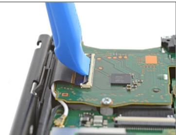
• Use an opening tool or your fingernail to flip up the small, hinged locking flap on the digitizer cable's <u>ZIF connector</u>.
