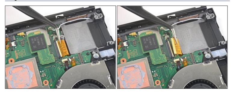
• Use a pair of <u>tweezers</u> to pull the ribbon cable straight out of its connector on the motherboard.
