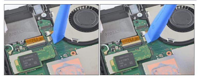
• Use an opening tool, spudger, or your fingernail to flip up the small, hinged locking flap on the fan cable <u>ZIF connector</u>.
