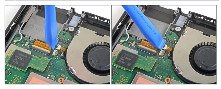
• Use an opening tool, spudger, or your fingernail to flip up the small, hinged locking flap on the power and volume button ribbon cable <u>ZIF connector</u>.
