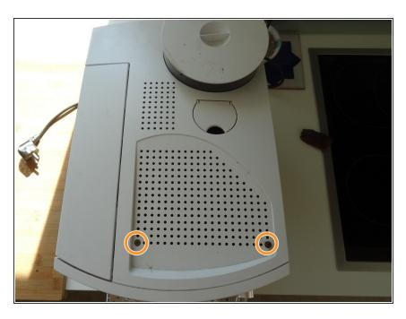
Remove the two Torx T10 screws on the top.
