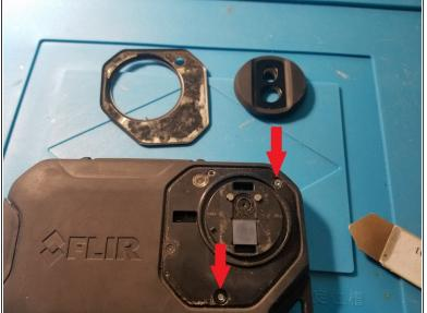
Using the iSesamo remove the taped on rear bezel and the clipped on camera bezel, then remove the two T6 torx screws.
