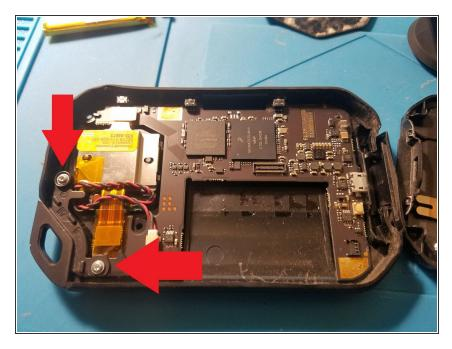
Once you have the device open and the screen disconnected, use the T6 driver again and remove these two screws holding the lanyard anchor in place, then you can carefully lift the motherboard out of its place.
