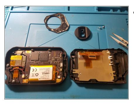
Be careful while opening, so you don't damage the screen connector or ribbon cable.
