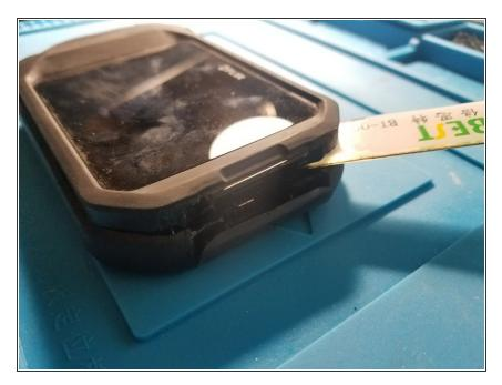
Once the screws are removed use the spudger on either side of the charge port, pop the clips open then you can work your way around to the other side of the body, although it will probably pop the rest of the way open once you unhook those clips.
