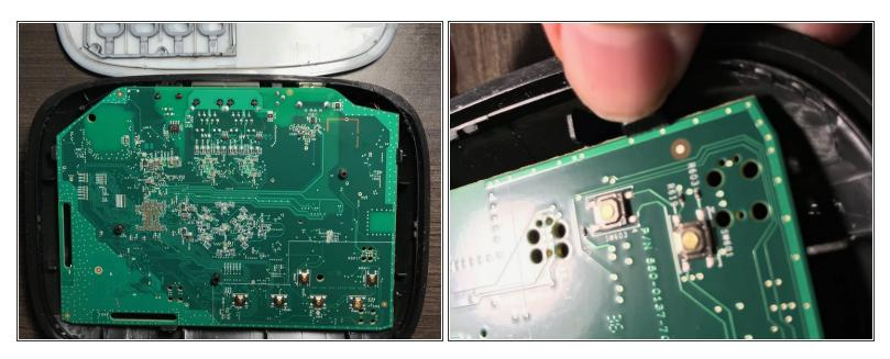
• Remove the lid. Inside there are three more clips holding the PCB in place.
