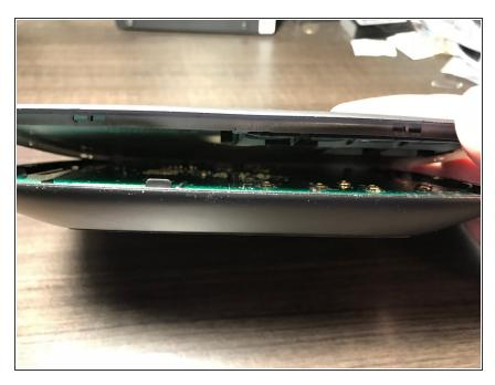
There are several clips fastening the top case on. Work your way around. Take your time. Once 3 sides are free, you can wiggle the top clips loose and remove the top case.
