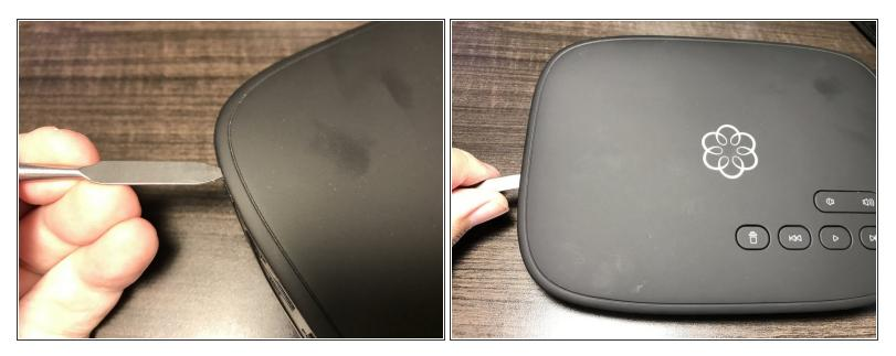
Use a tool to slip between the seam and release the clips holding the top case on.
