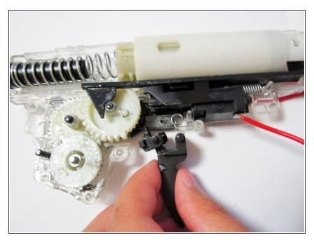
• Pull the trigger off the gearbox.
