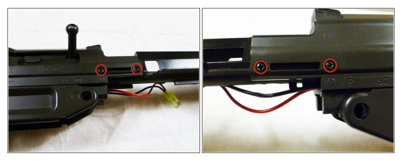
Using a Phillips #1 screwdriver, remove the two 8mm screws above the hand guard on both sides of the gun.
