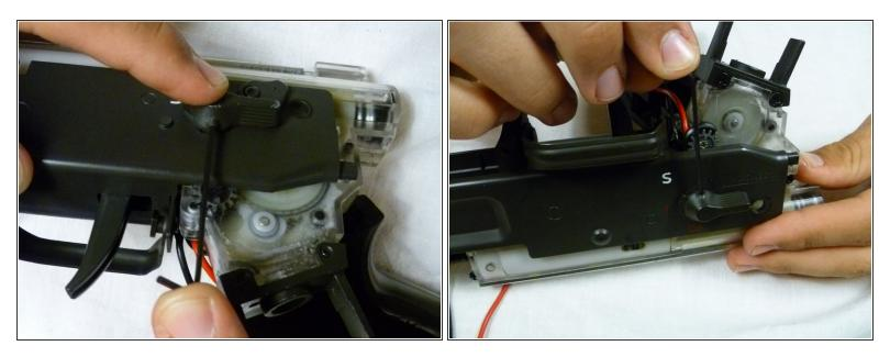
Using a small allen wrench, carefully unscrew the screws holding the safety switch in place on both sides of the gun.
