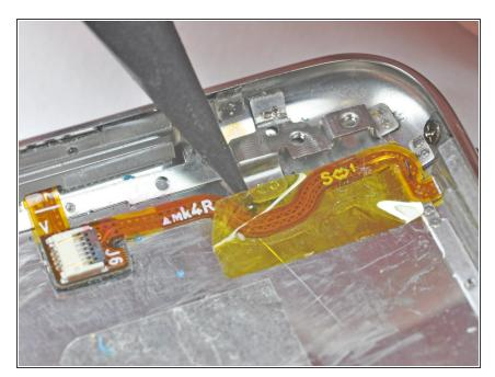
• Use the tip of a spudger to remove the yellow kapton tape covering the power/volume control ribbon cable.
