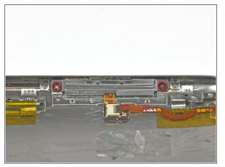
Remove the two Phillips screws securing the power/volume controls to the rear panel.
