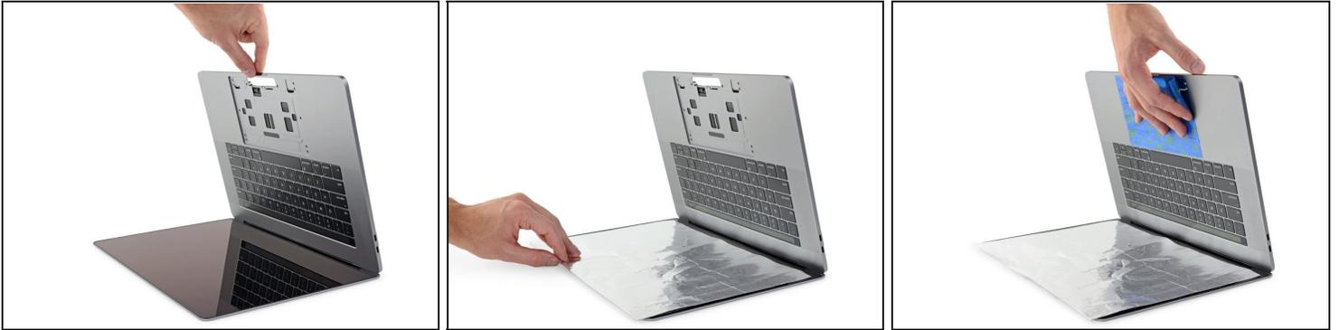
**⚠** The liquid adhesive remover provided in your kit can damage the antireflective coating on your MacBook Pro's display, as well as the plastic keyboard keys.
