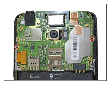
Remove the two 4 mm Phillips screws securing the motherboard.
