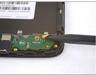
Use the point of a spudger to pry up and disconnect the antenna cable from the daughterboard.
