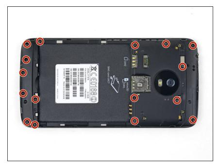
Remove the sixteen 3 mm Phillips screws securing the motherboard and daughterboard covers.
