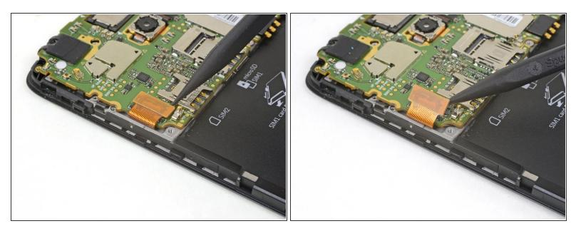
• Use the point of a spudger to pry up and disconnect the display connector from the motherboard.
