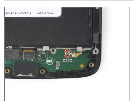
Remove the 3.4 mm Phillips screw securing the daughterboard to the frame.
