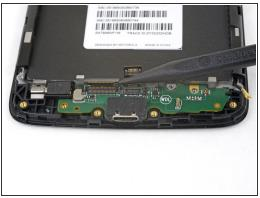
Use the point of a spudger to pry up and disconnect the two flex cable connectors from the daughterboard.
