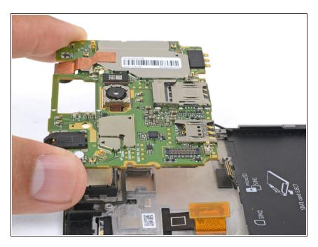
Lift up and remove the motherboard.
