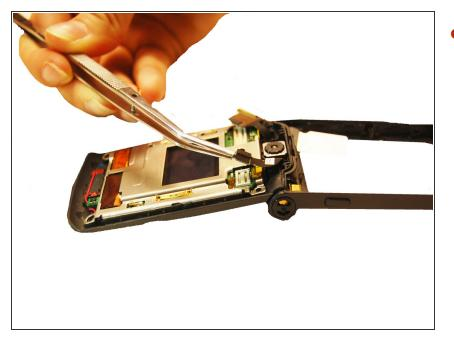
Once the screws and upper casing have been removed, locate where the camera attaches to the upper circuit board and detach it using a pair of tweezers.
