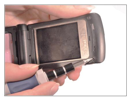
Use the Torx T5 screw driver head to remove the four 5.4 mm screws from the upper inner face.
