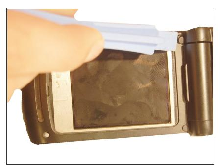
• Use the blue plastic opening tool to pry off all four of the rubber stickers from the upper inside face.
