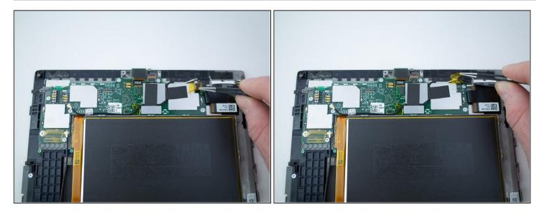
• Grab the yellow tape with a pair of <u>tweezers</u> and pull upwards to disconnect the pressfit connector.
