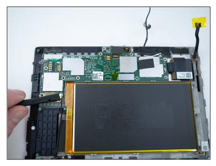
Use a spudger to disconnect the second antenna cable from the motherboard.
