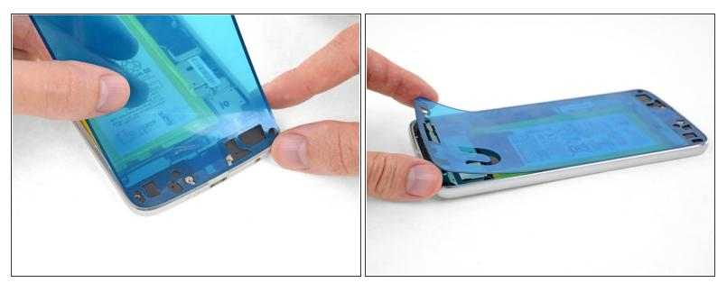
Hold the adhesive sheet with the exposed adhesive facing down, and carefully align it into the lower edge of the phone.
