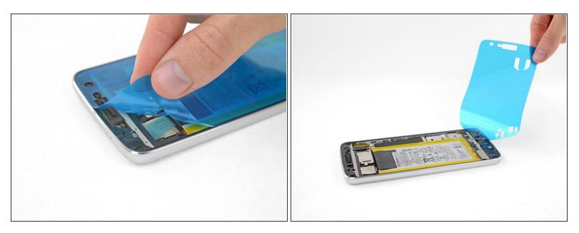
• Peel off and discard the plastic liner, exposing the display adhesive.
