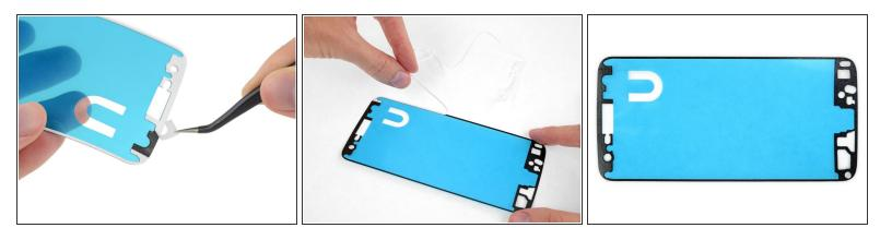
• Peel off and discard any remaining paper liner, exposing the adhesive on one side.
