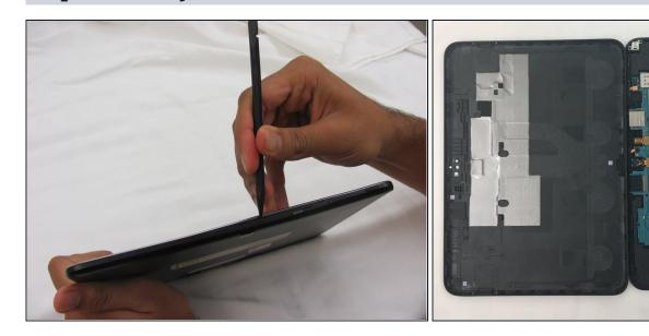
• Insert the wedge of the nylon spudger and slide it between the front and back panels until the back comes off.
