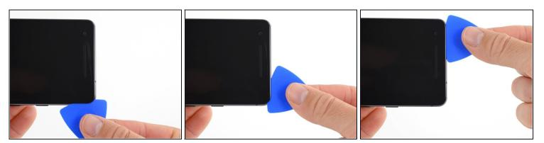
• Slide the opening pick around the upper-right corner and along the top edge of the phone.
