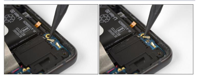
• Use the tip of a spudger pry the black antenna cable connector straight up and disconnect it.
