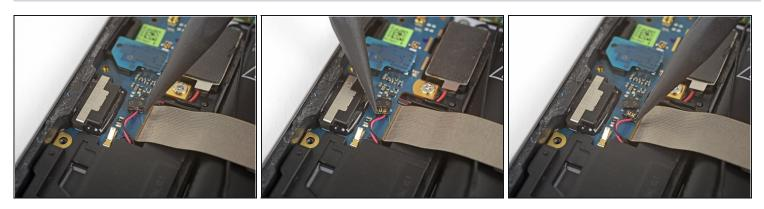
• Use the tip of a spudger to gently push the speaker cable connector out of its socket horizontally, alternating pushing either side of the connector out a little bit at a time.
