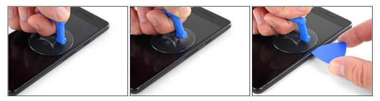
• Pull up on the suction cup with firm, constant pressure and insert an opening pick between the front panel and rear case.
