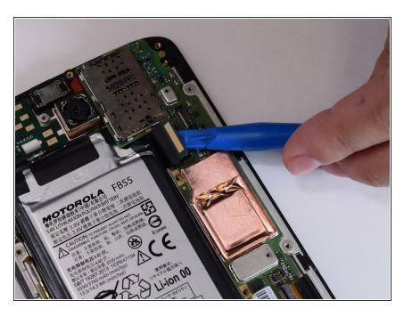
Using a plastic opening tool, unlatch the small black ribbon on the upper right corner of the battery.
