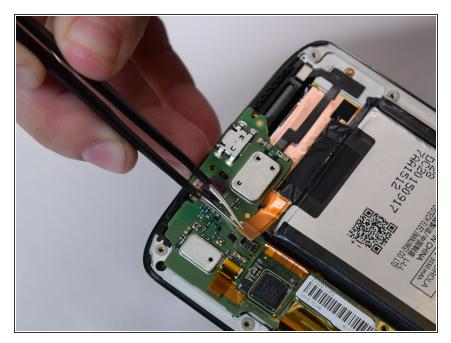
Use the angled tweezers to disconnect the small connector near the bottom right corner of the battery.
