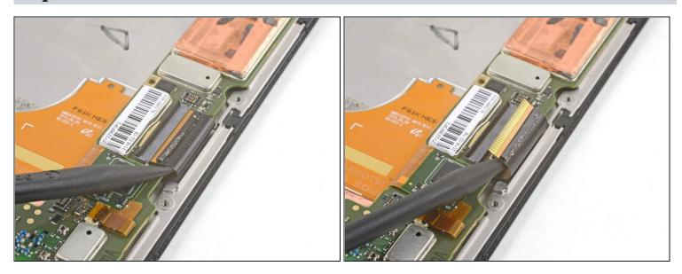
• Use a spudger or <u>tweezers</u> to walk the flat cable out of the ZIF connector.
