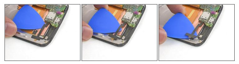
• Insert an opening pick underneath the flat flex cable and slide it to free the cable from the frame.
