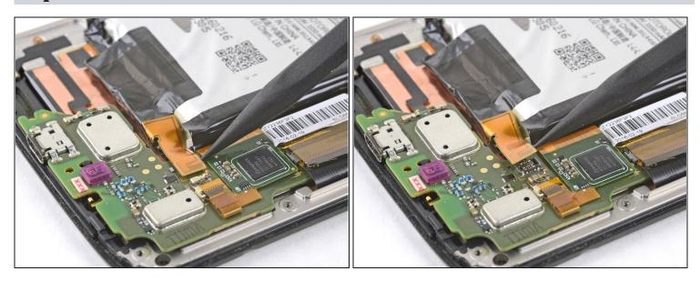
• Use the point of a spudger to pry up and disconnect the battery pack connector.
