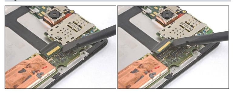
• Use the flat end of a spudger to pry up and disconnect the accessory module connector.
