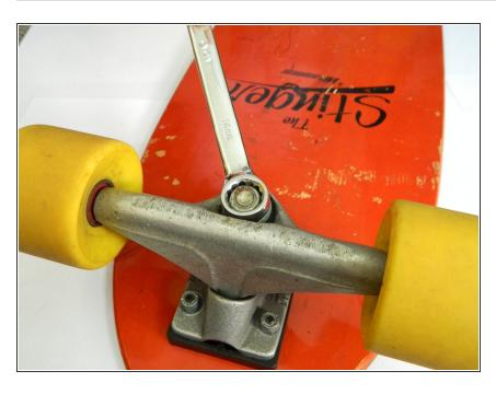
Place the washer back over your new kingpin bushing and thread on the kingpin nut to your preferred tightness. This harder bushing will make it harder to turn, preventing the wheels from hitting the deck on hard turns. To remove your risers, simply remove your trucks following the reverse directions of the <u>Truck</u> <u>Installation</u> guide. Follow steps of this guide in reverse to replace your old kingpin bushing.
