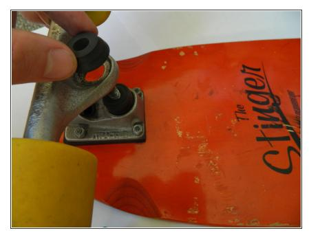
Another way to further prevent wheel bite is to replace the kingpin bushings with a harder ones. You will first want to remove the kingpin nut completely using your 9/16" wrench.
