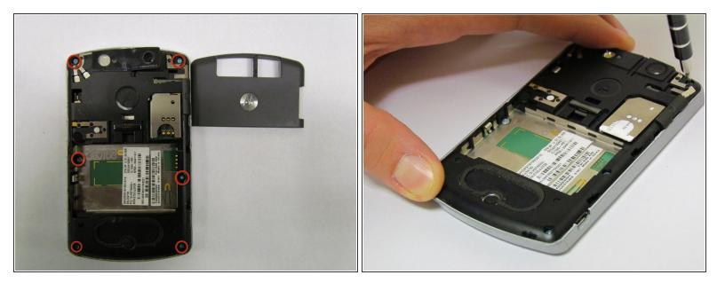
• Remove the six labeled screws with a T5 torx screw driver.
