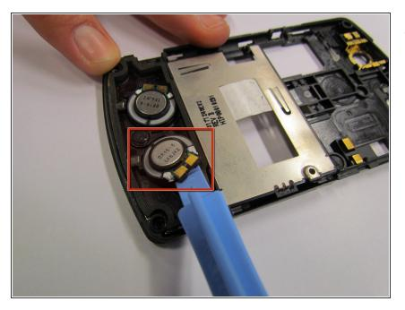
• Remove the speakers by using the plastic remover tool.
