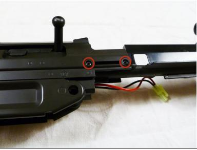
Using a Phillips #1 screwdriver, remove the two 8mm screws above the hand guard on both sides of the gun. There should be four total.
