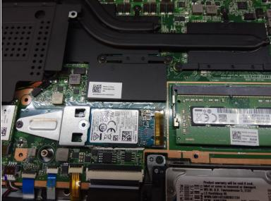
The motherboard on the 330s with a GTX 1050 discrete graphics card is different than the motherboard on a 330s with integrated UHD graphics. Upgrading the graphics card is not possible, unless you can get a useable motherboard from a "for parts" 330s, then (in theory) it could be possible. I have not been able to test that myself in practice.
