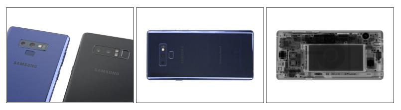
Another subtle (but good) change: the fingerprint sensor has packed its things and moved to a happier location, south of the rear camera.
