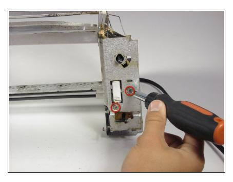
Remove the two Phillips #4 1 cm screws that were under the faceplate.
