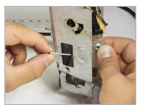
Remove pin holding the On/Off switch in place.
